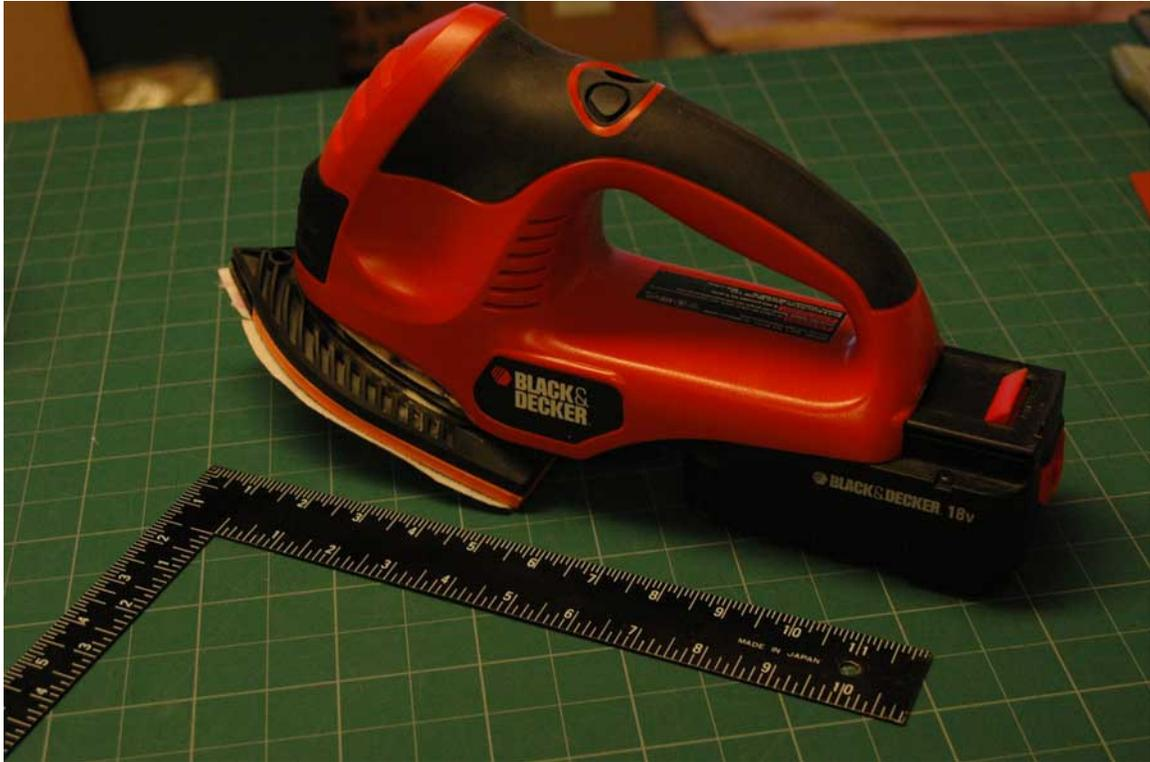
**My cordless power tools use nickel-cadmium batteries. On the downside, they are very hard to find in the sizes needed to power an electric car, more expensive than lead, very toxic, and not as easy to recycle.**
