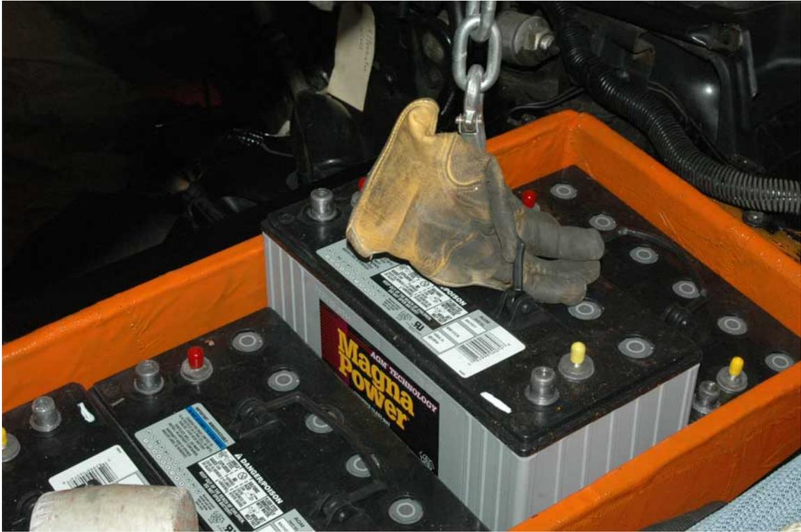
**Not knowing what else to do, I gave the battery a sideways knock with a rubber mallet. Instantly the Vette fell away from the battery. I could stop sweating bullets.**
