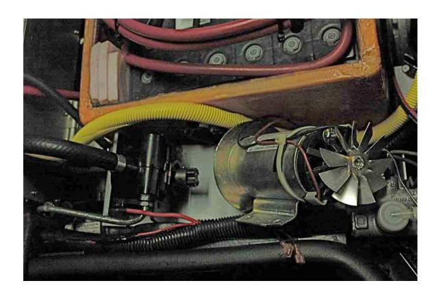
I noticed that the tail shaft of this type motor was probably designed to hold a fan blade, probably to cool the motor. Spend a lot of time looking for small fan blades. Spend still more time getting the thing properly mounted. But that presents a new problem. Bare metal blades spinning at 5000rpm could do bad things to nearby wiring.
