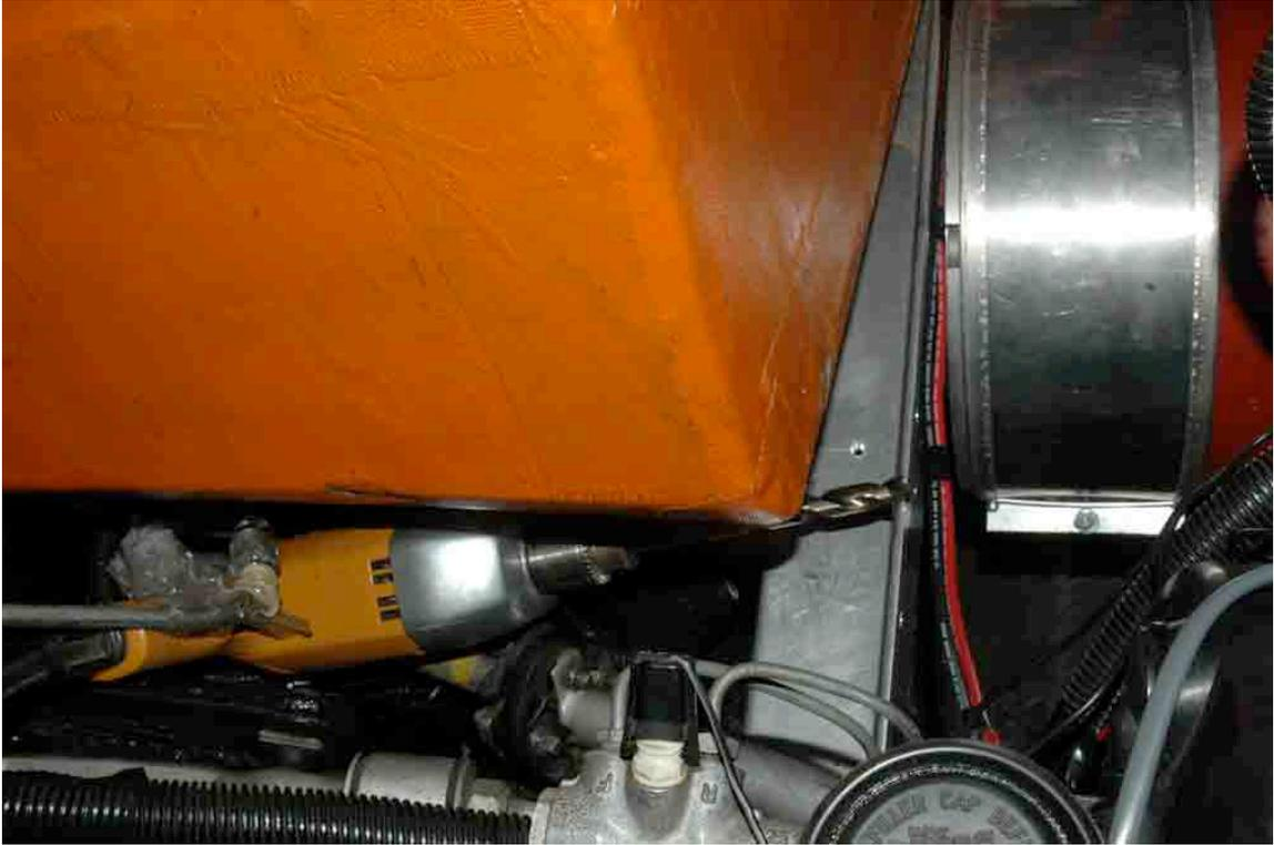
The steering fluid tank is removed and the middle battery box is tilted out of the way. This gives me just enough room to bring in a hand drill. I drill and countersink-mounting holes in one of the battery box supports. Next, I make a bracket to bolt on to the bracket that holds the power steering unit.
