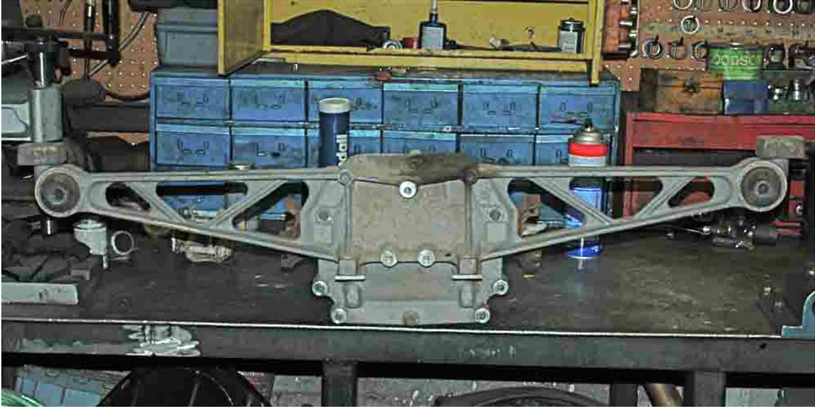
As you can see in this photo, the Corvette differential has “bat wings” that form part of the car’s frame.
