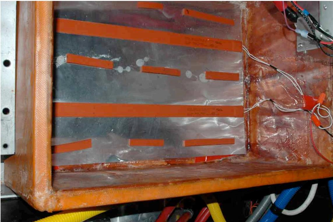
After placing the sheet at the bottom of the battery box, silicone rubber spacers are put in to support the weight of the lead batteries. Once I had the batteries back in the box, I started testing. The new system easily passed the smell test, and after resetting the temperature sensor, it finally looked like I could move on to the next chapter.
