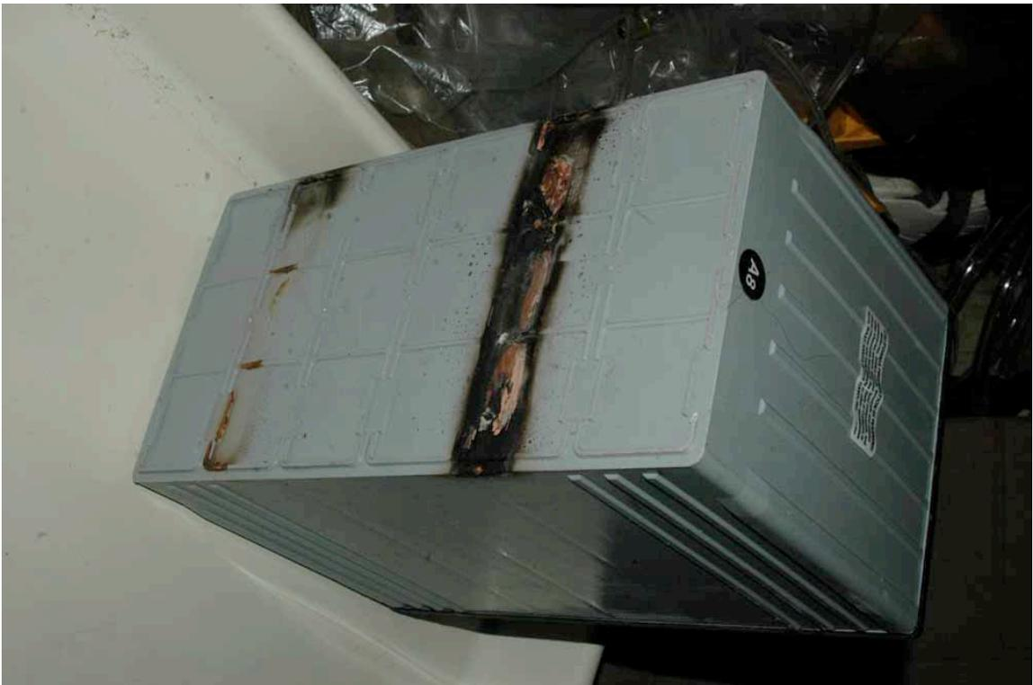
And some of the batteries showed signs of melting. Poor heat flow!
