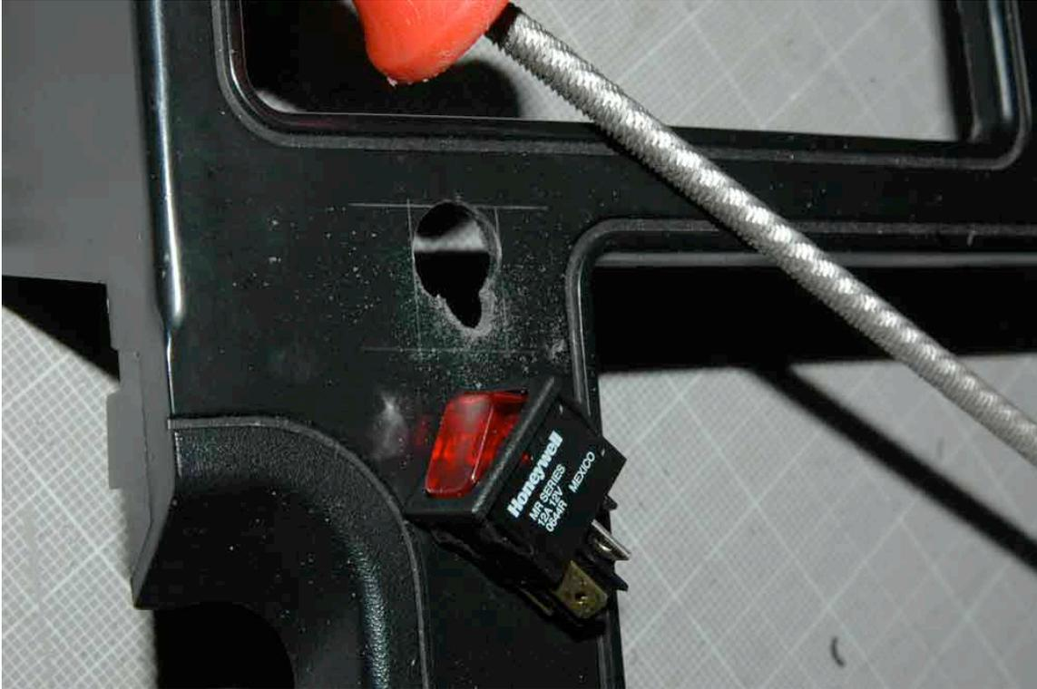
I carefully drill a hole in the plastic; then draw lines that are the same size as the switch. Using some small hand files very slowly, I shape the round holes into square holes of exactly the correct size.
