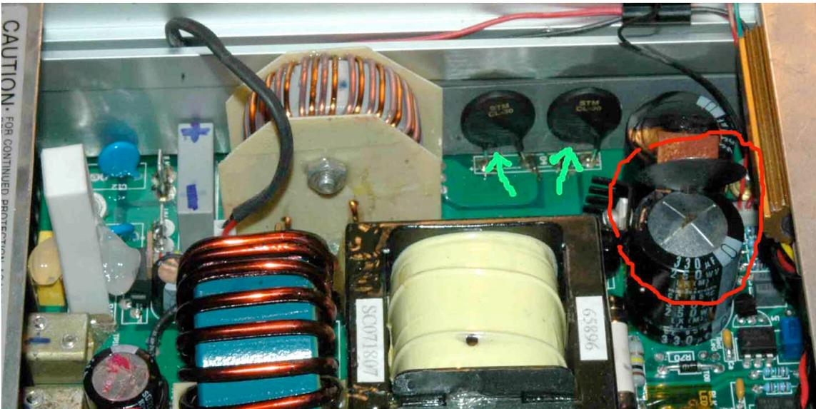
In the photo, I have circled the dead capacitor. The arrows point to the “in-rush limiters” that failed to protect the capacitor. At least it didn’t explode again.
