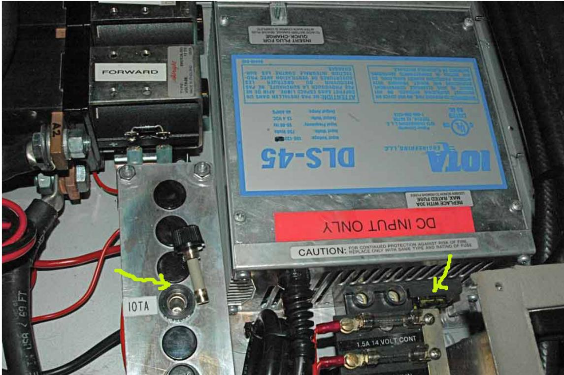
This photo shows the unit in place, inside the waterproof Zilla box. Arrows point to the fuses that were designed to protect the converter from power surges.
