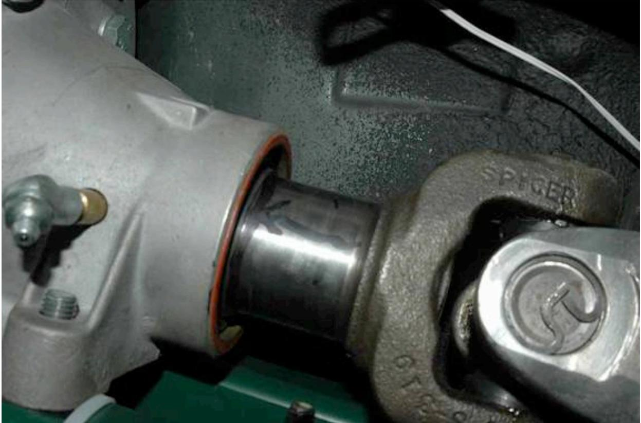
The slip yoke should slip into the motor bell housing where it discreetly, but firmly, mates with the armature shaft. Away from prying eyes, foolish hands, and flying stones. But as the driveshaft “shrank” the yoke slipped too far out of the bell housing as you can see in the photo above.
