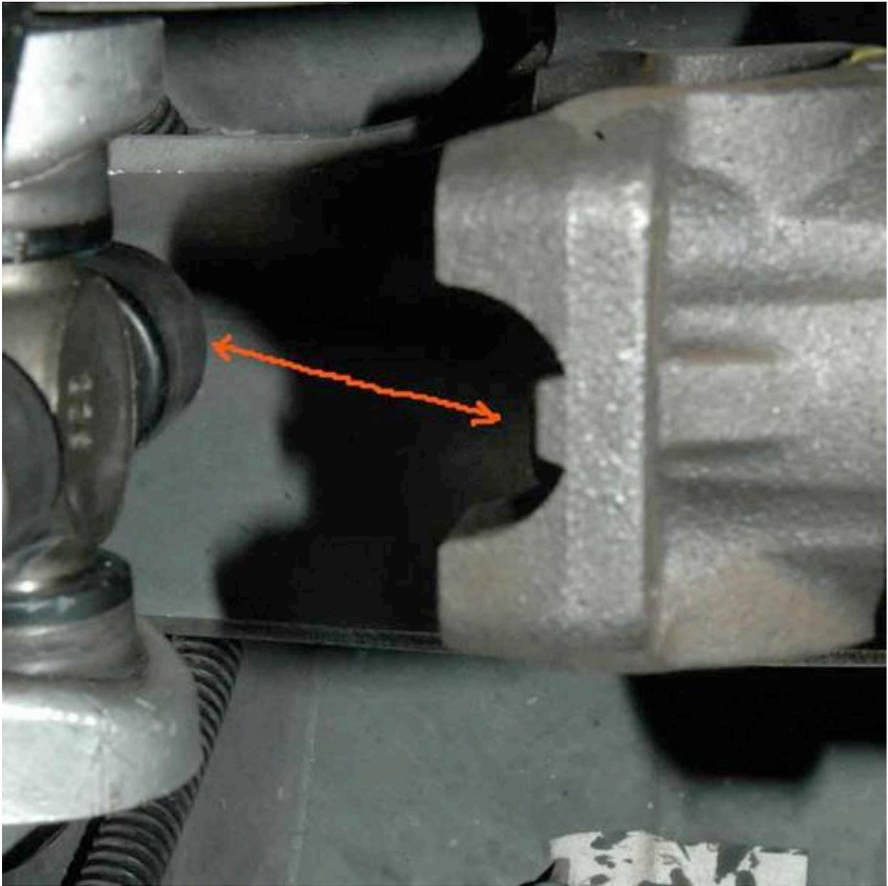
Instead of asking the shop to make a new shaft 43.25 inches long, I give them the present shaft, and order a new driveshaft that is 1.62 inches longer.
