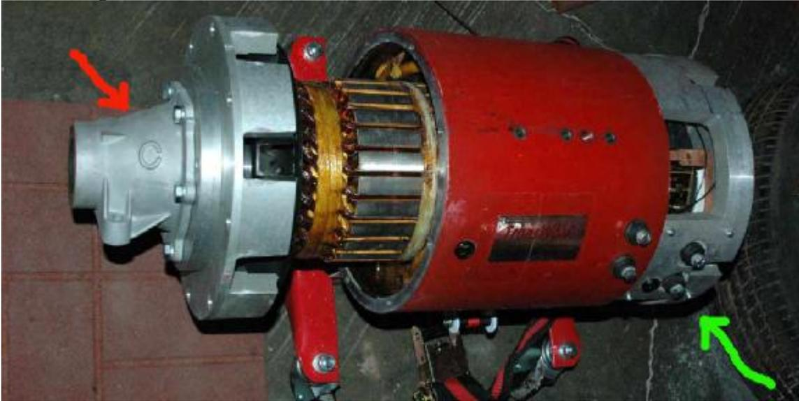
In this photo, the red arrow points to the bell end and the green arrow points to the end that should hold the washer!
