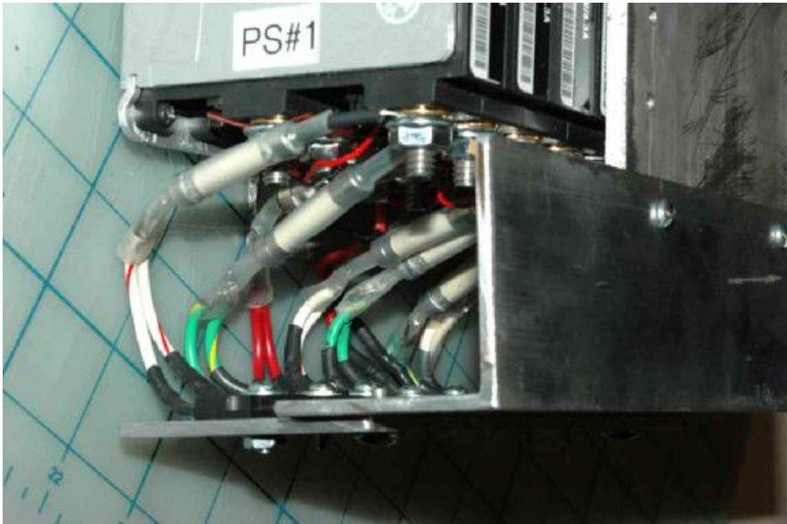
I had mounted the metal diode plate to the Vicor metal bracket. Chris told me to rebuild the converter in such a way that the diode plate would be properly grounded, but without any metal to metal contact with the Vicor.
