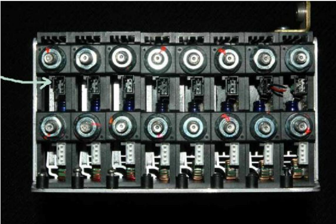
Each power module will need a tiny resistor plugged into a tiny socket, found at the output end of the Vicor. (see photo above)
