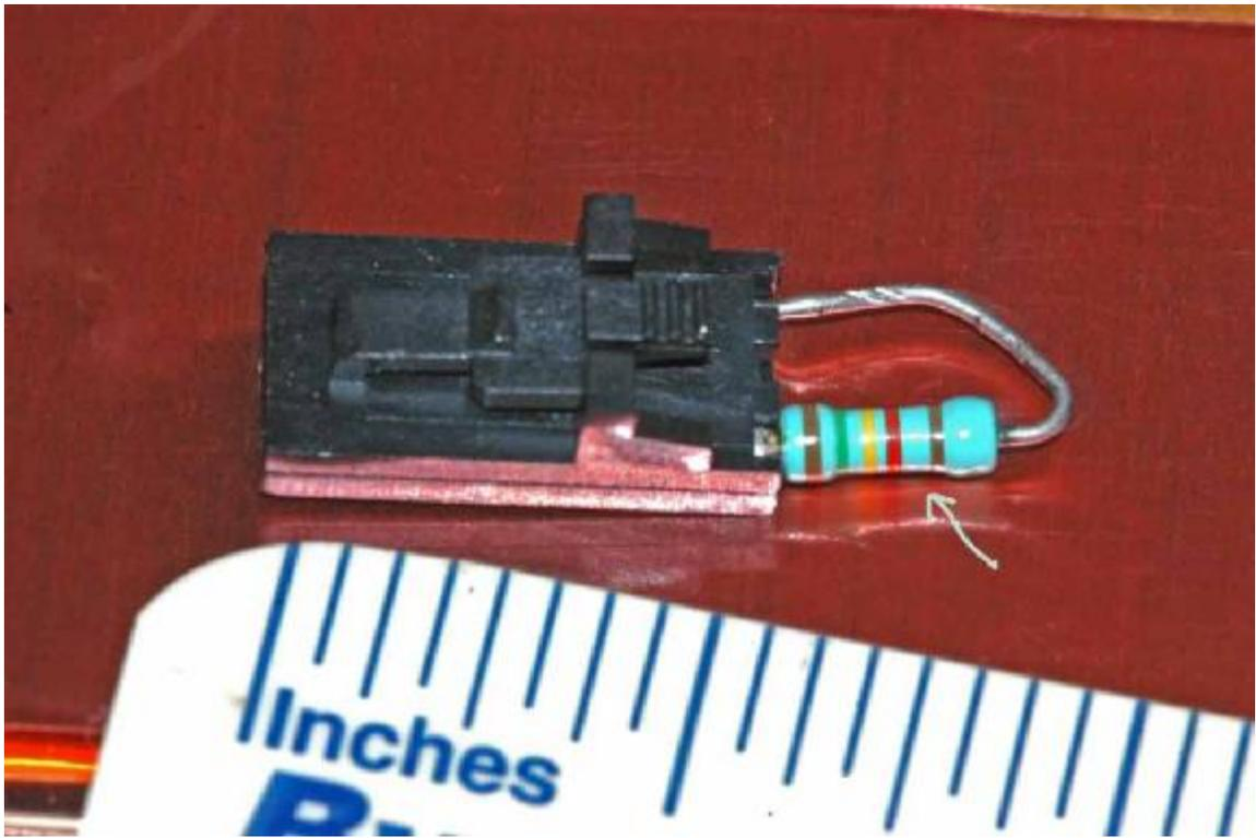
In this photo you can see just how small the resistors are. The color bands form a code that tells an electrical engineer what kind of resistor he or she is dealing with.
