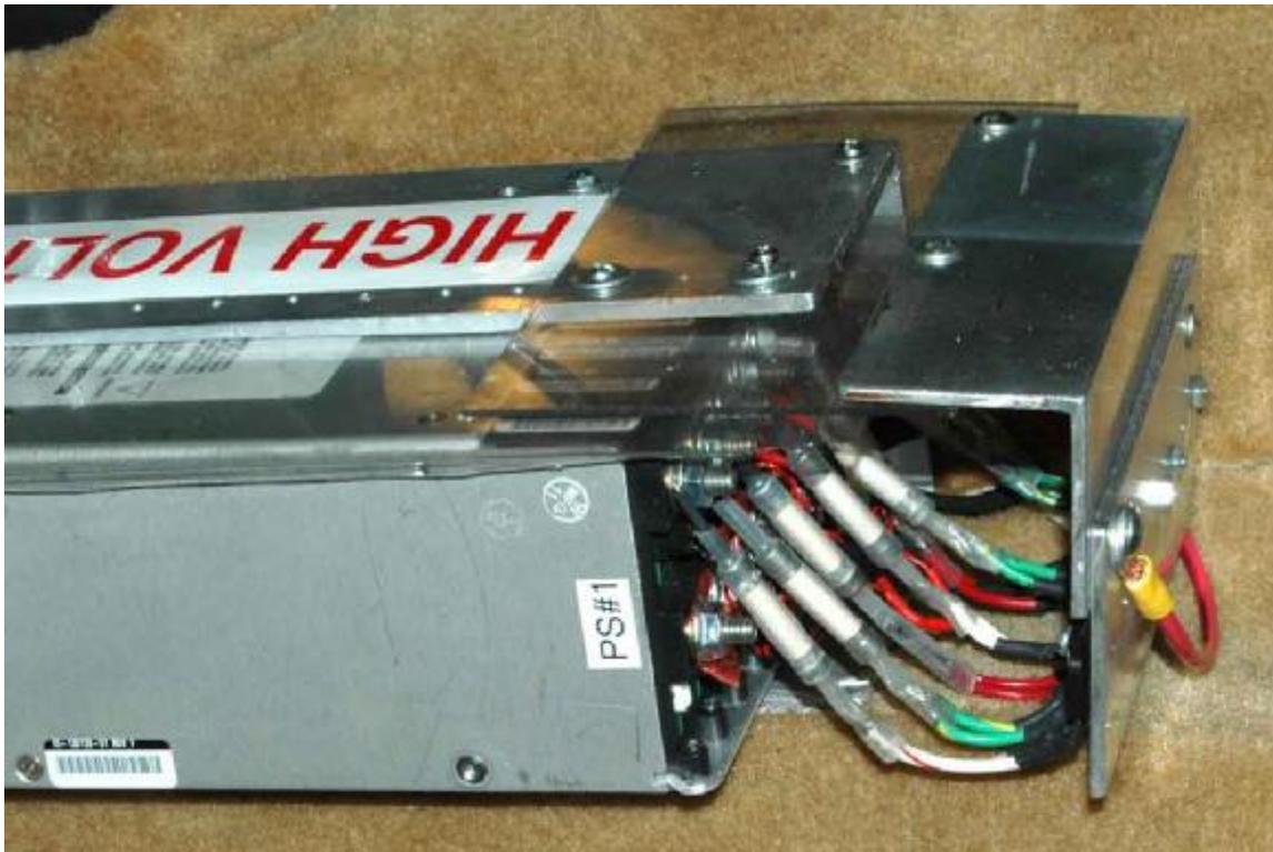
I cut a piece of clear plastic and attach the diode plate to it. Then I made certain that the plate was well grounded.
