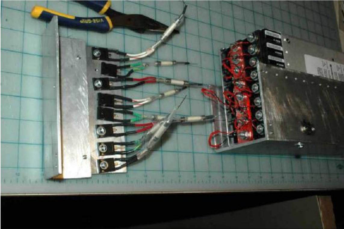
Chris has me add diodes and fuses. I also use heat shrink tubing to keep bare wires from shorting out. The diodes are all bolted to a metal plate, which acts as a heat sink, keeping the diodes from getting too hot.
