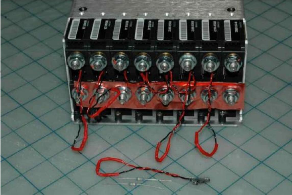
Chris puts together all the plugs and resistors and covers the resistors with heat shrink tubing.
