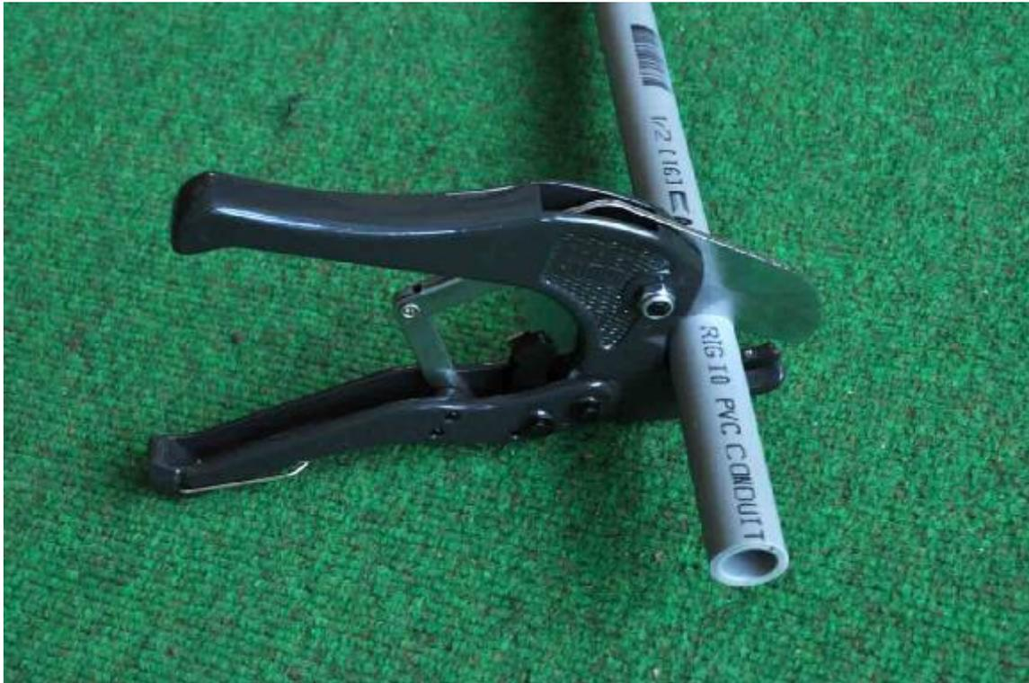
I normally use a hacksaw to cut pipe, but I discover a plastic pipe-cutting tool makes a cleaner, burr free, cut.
