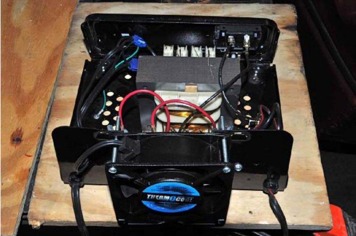
I bolt on a muffin fan to the back of my charger. With plenty of cooling air, the charger can run all day.
