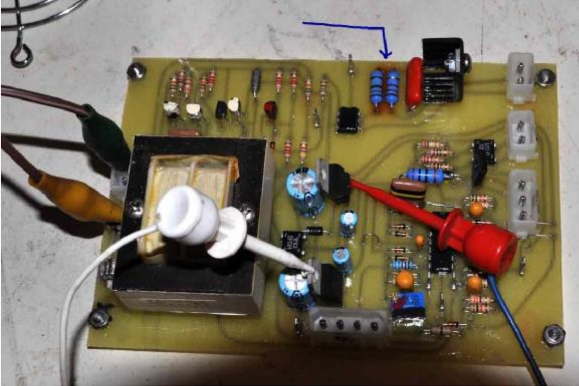
On the circuit board, we find 2 diodes that overheated and burnt the board. Problem solved!
