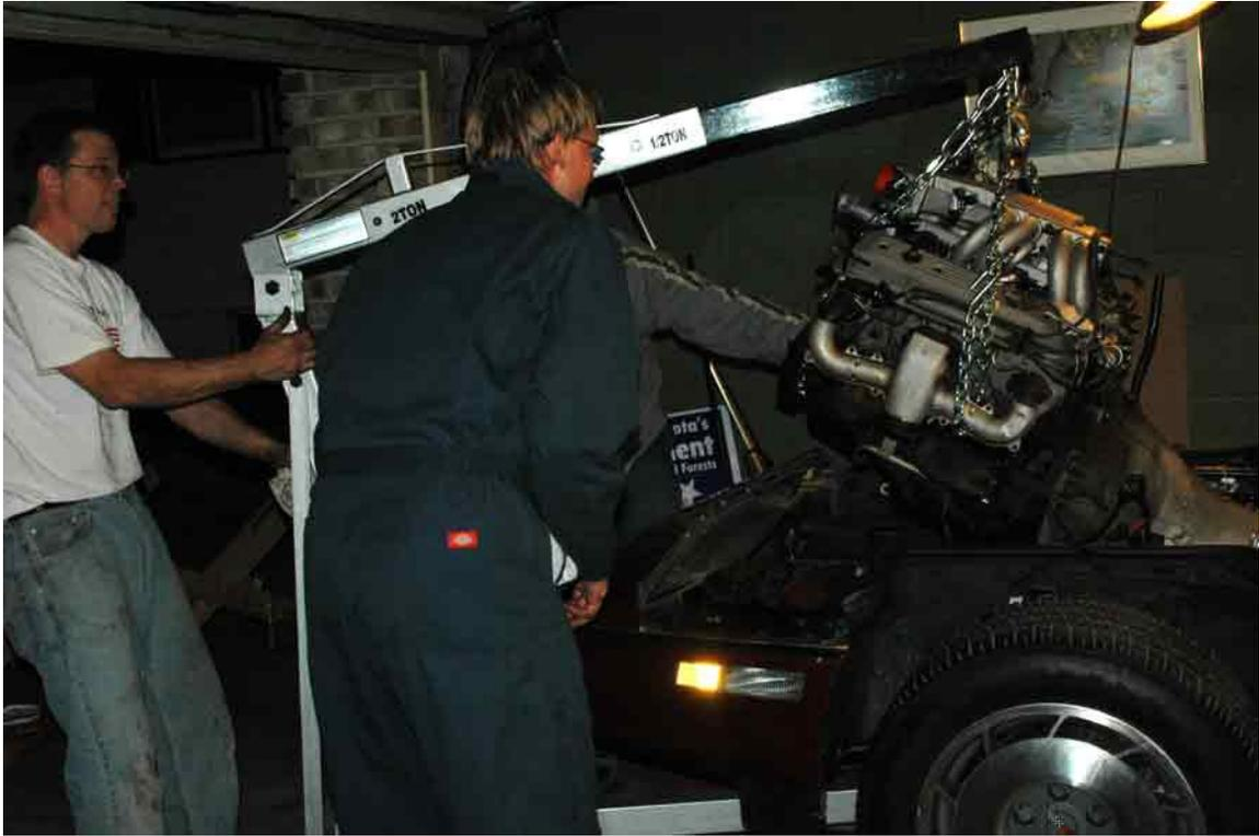
**Brad got rid of the load leveler and had me remove my eyebolts. With the help of Jim and Phil, Brad placed the hoist to one side of the car and wrapped chains around the engine. The hoist was connected to the chains; and the last engine mount bolt was removed.**
