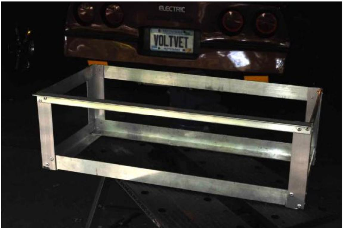
**I have what is needed, an aluminum, open-sided box that can keep the lithium straight, level, and in its place.**
