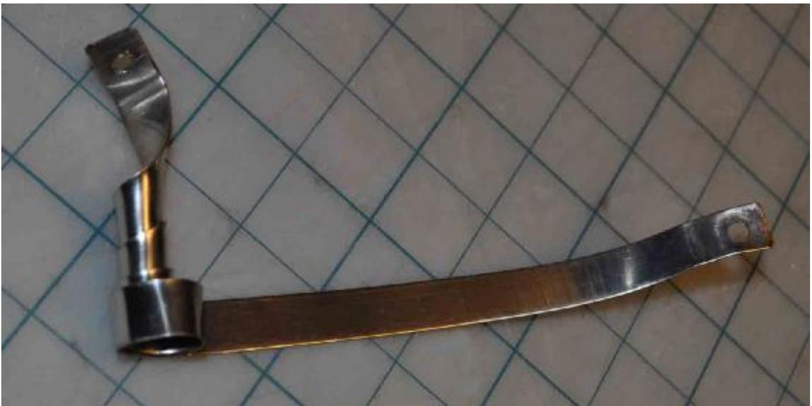
But, drilling screw holes in thin stainless steel proves to be very dangerous! The stainless steel wants to grab the drill bit, twist itself up and hit my hand.
