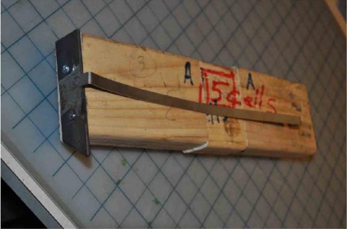
Chris Simon builds me a bending jig exactly the right length for making longer 5-cell straps.
