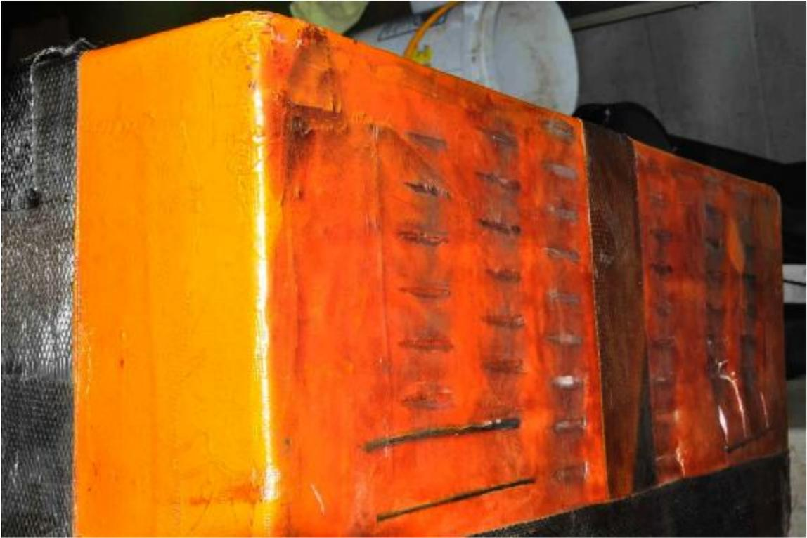
After 5 years, cracks had appeared on the bottom of the old fiberglass box. To keep that from happening again, I made the bottom of the new box twice as strong as the old,
