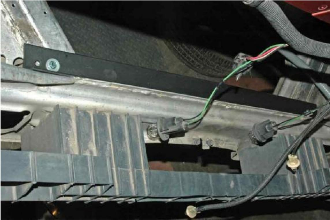
The angle iron that supported the rear edge of the battery box is now replaced with a wider piece of angle aluminum for better support.
