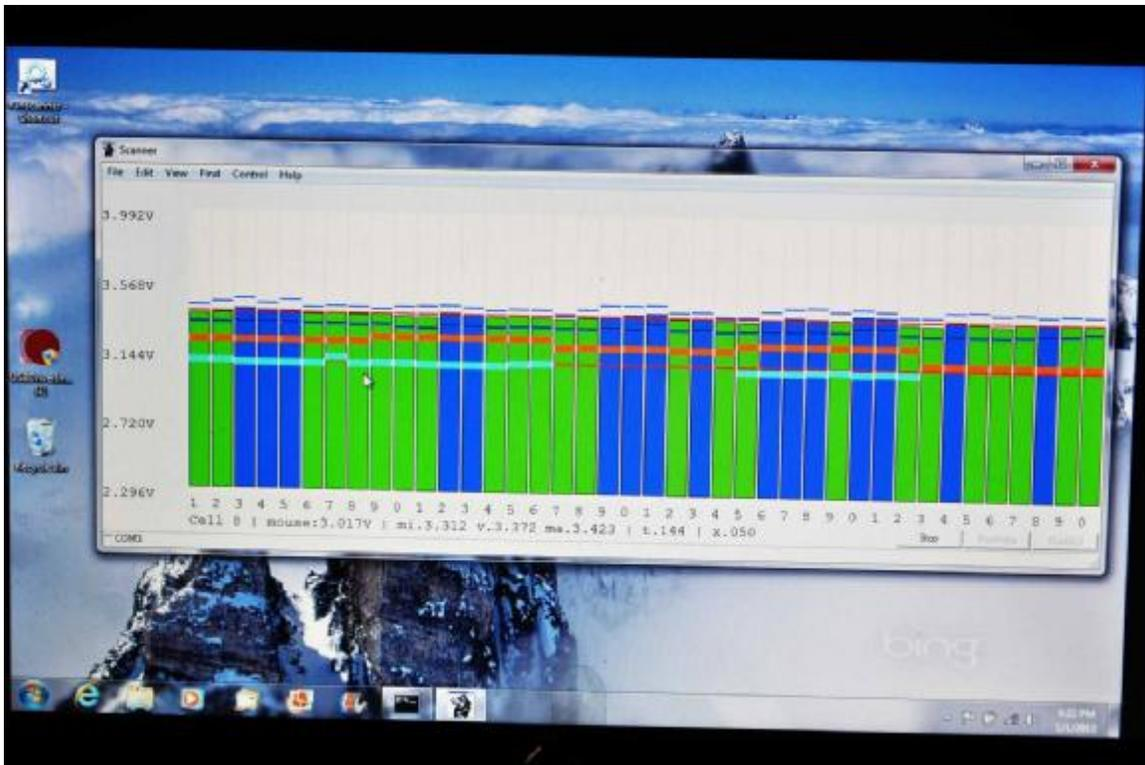
The boards can display a graph, on my laptop, showing the condition of each cell.
