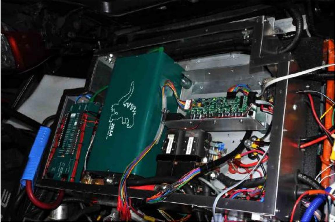
I put the electronics box back in place and put the 5<sup>th</sup> regulator board inside.
