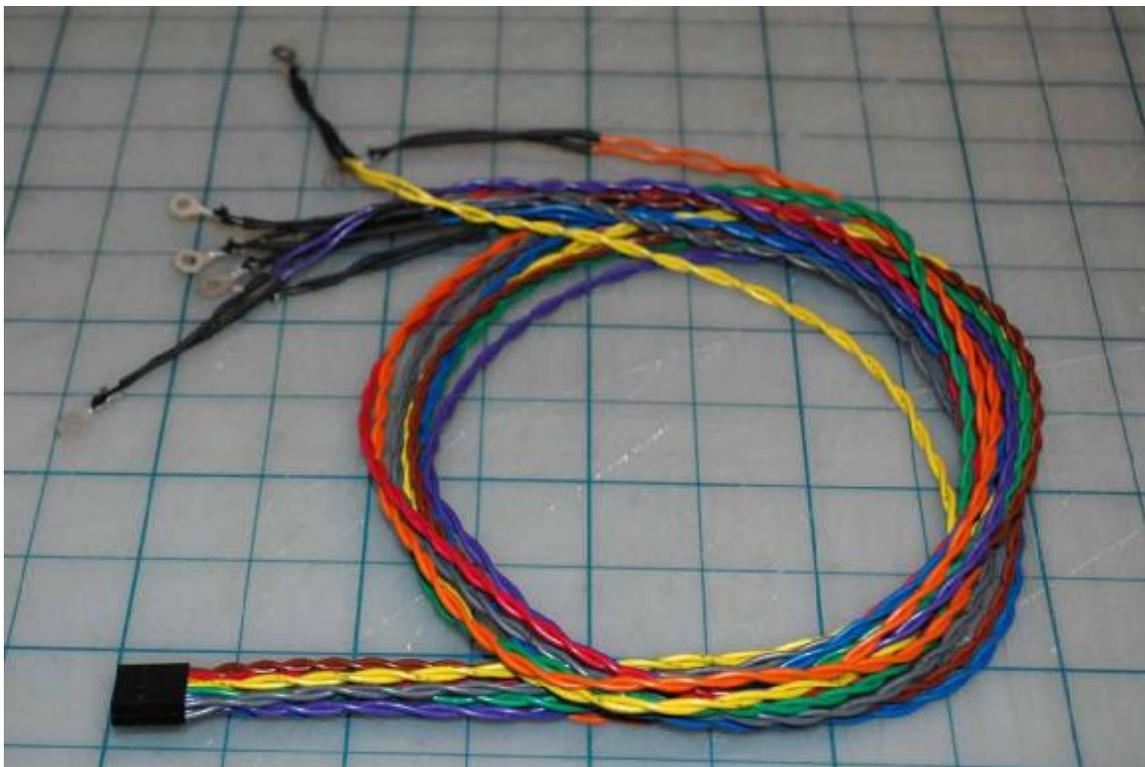
**I ever so carefully soldered the tiny sensor leads to the braided wiring harness.**
