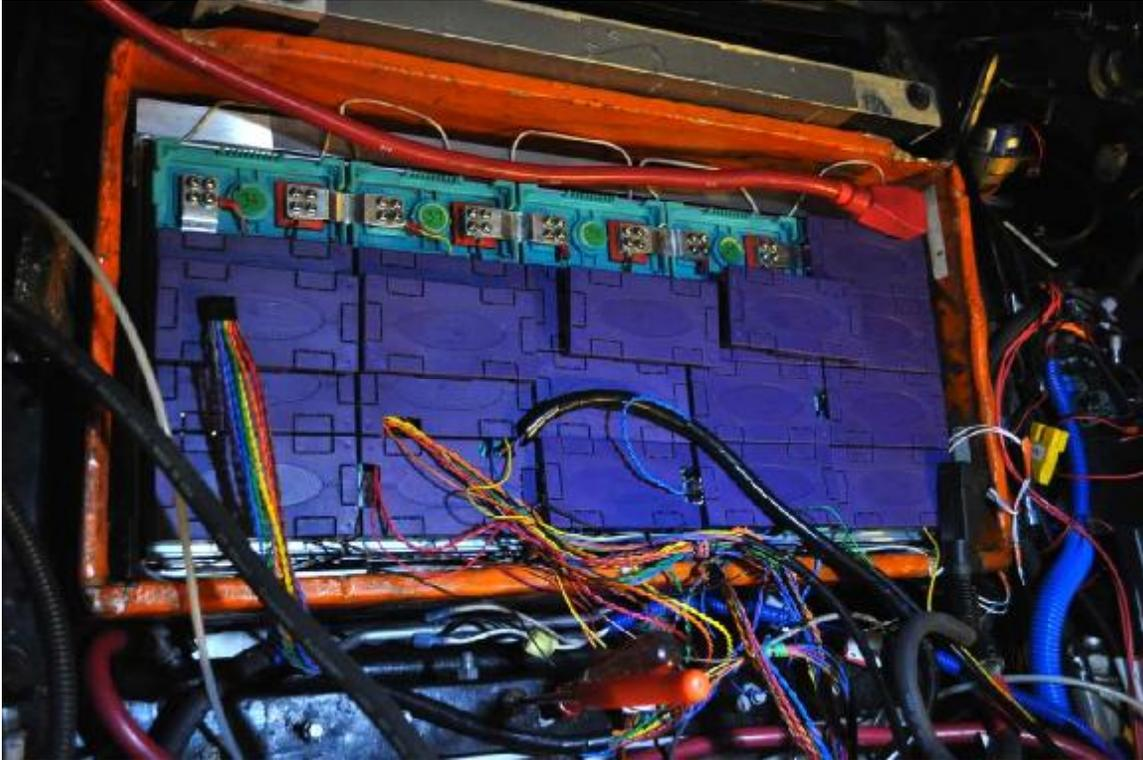
So I redid all the buss bars and wires. Hopefully now I'm finally finished with the front box.
