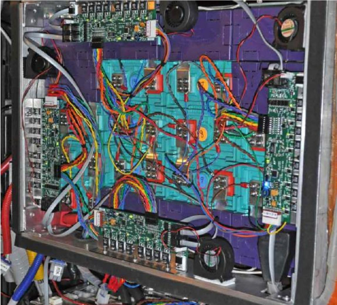
But not quite cool enough! If the boards get to 180 degrees they will switch off to keep from burning out. With my computer showing some of the boards reaching 160, I install a Manzanita cooling fan for each board.
