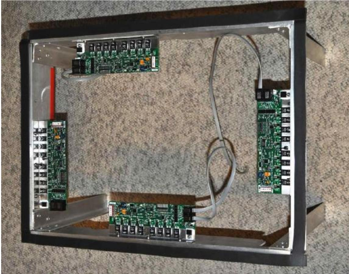
Next, I attach 4 boards near the top of the frame.
