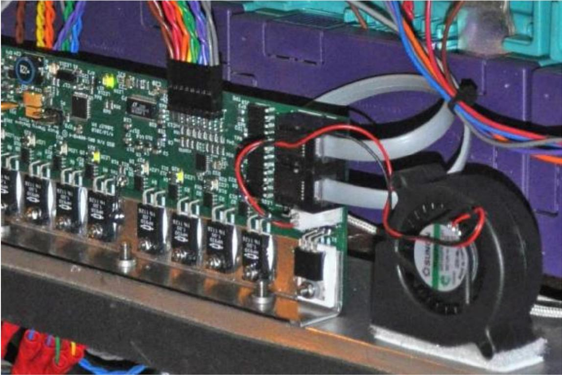
**These are 9 speed fans that plug into the boards. The hotter they get, the faster the fans run. If I like, I can also command the fans to run at a speed of my choosing. In any case, I no longer have to worry that the boards will overheat.**
