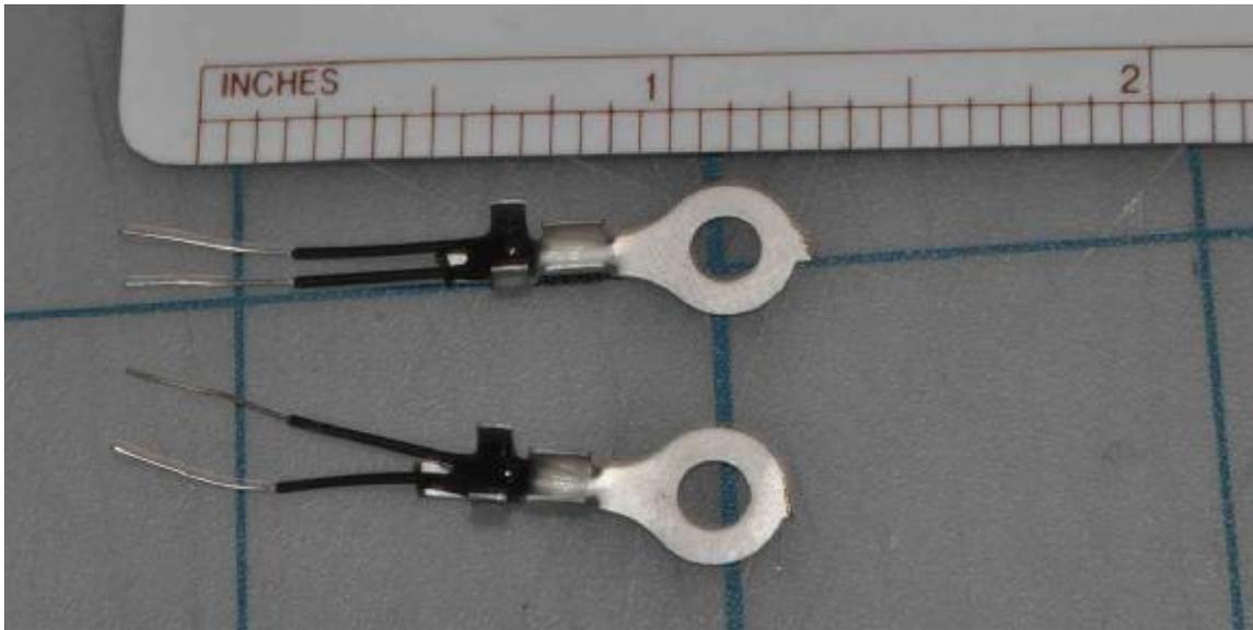
**I finally decided to super glue each sensor to a metal ring terminal. After that**
