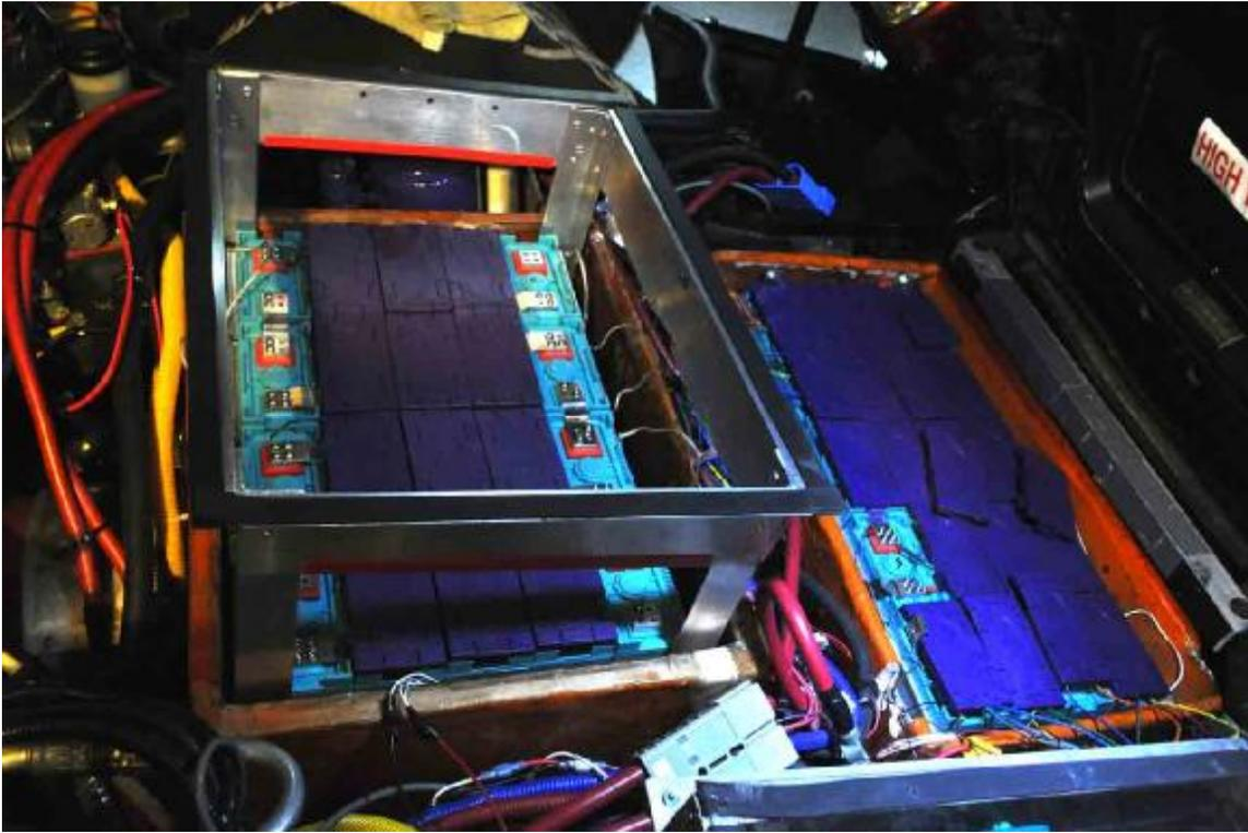
For this purpose I make a metal frame that slips into the middle battery box.
