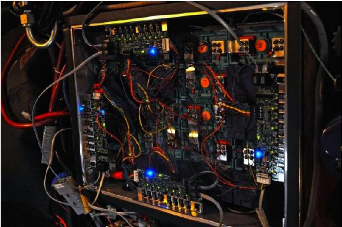
With every thing finally wired up you can see that the regulators put on quite a light show. The blue LED light flashes when the board is communicating with a computer. The green light next door indicates that the board is operating correctly.
