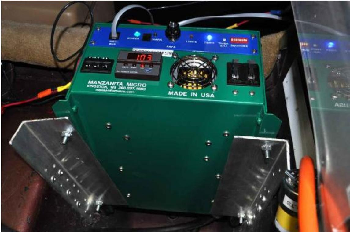
**This charger will run on either 110 or 220 volts and charge up any battery pack from 12 to 450 volts. I pay for the optional push button voltage output gage and the expensive multimeter. I also pay extra to have this 20 amp charger beefed up to 30 amps.**
