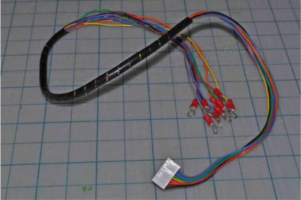
The volt sensor wires get a different style ring terminal that is attached to the negative post of each cell.
