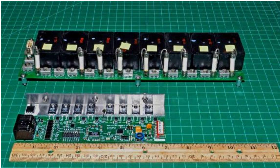
As you can see in the photo above, the Manzanita regulator boards are much smaller than Lee's, but do not have the big fuses for protection against unforeseen problems. Instead, Manzanita boards have something called a poly fuse, which is rated at only 50 milliamps (my cell phone battery is rated at 1,200 milliamps).
