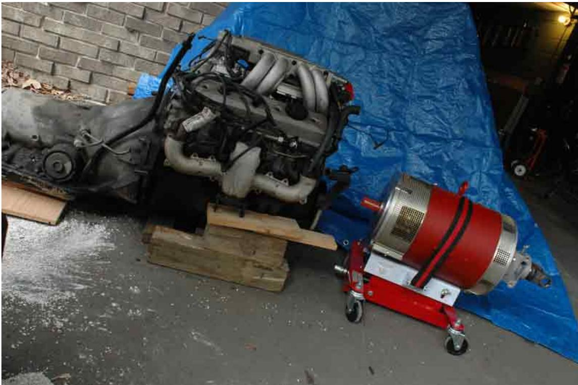
V8 Engine and transmission next to electric TranswarP motor
