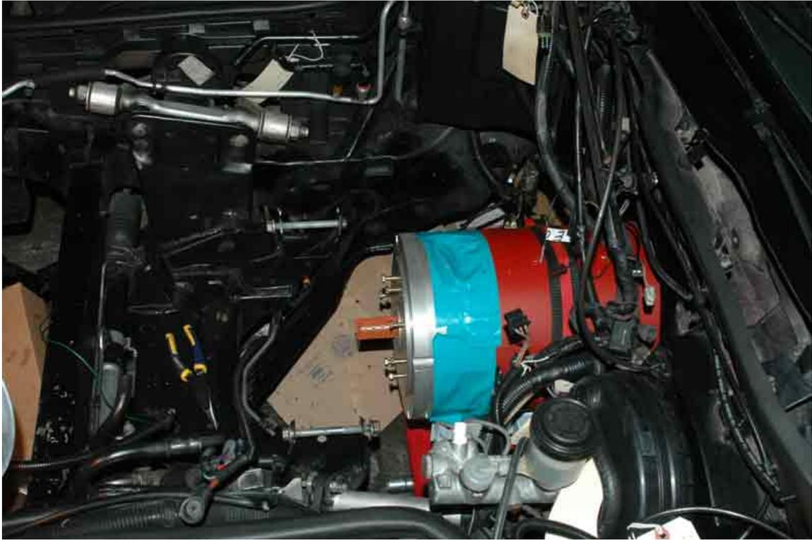
**Also, by moving the motor forward, we can bring the WarP closer to the original engine mounts and all that steel that recently held up a big V-8.**
