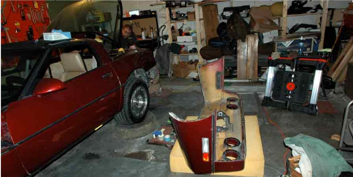
**With the gas tank finally in full view; the end of the job was in sight. But, no. Even after cutting away the steel straps holding the tank to the frame, the tank could not be removed.**
