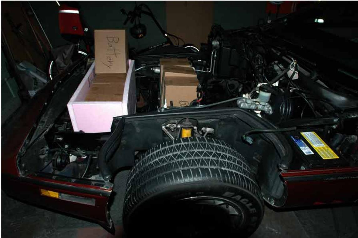
**The original Corvette battery is to be used as the 14<sup>th</sup> battery in the electric car and stay in its original compartment, as you can see in the lower right of this photo.**
