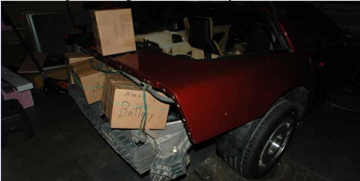
Now the batteries. As a general rule it's not a good plan to put all your batteries in one basket. You want spread the weight while keeping the batteries between the front and rear wheels. This is so you don't mess up the cars handling.
